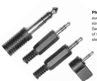
**Phone plugs** (also called jack connectors or audio jacks) are available in a number of different sizes. Mainly used are "Mini Jack Plugs" (3.5 mm) or (larger) "Jack Plugs" (6.3 mm). One ring (at the top of the plug) indicates a mono connection, two rings a stereo connection.
